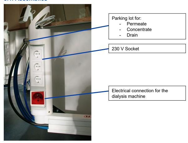
Grounding, dialysis machine connection and electrical sockets for the French version:
